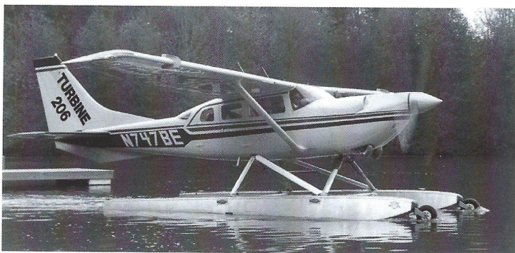
FIGURE 7. Soloy Turbine Powered 206 EDO 3500's Demonstrating Low Speed Taxiing.
